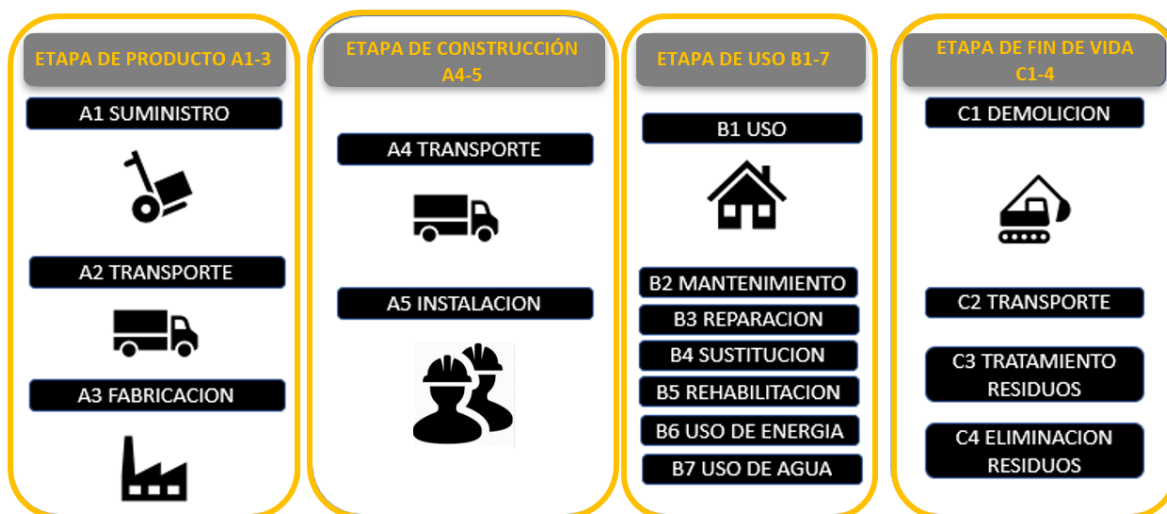
Figure 2: Stages of the life cycle of a product according to the analysis "from the cradle to the grave".
